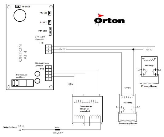
Appendix G – Typical Wiring Diagram, 1 Heater, 1 safety relay
