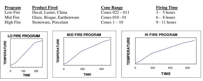
Note: the Conefire Programs can be removed from the controller selections. To disable a program set, see the configuration appendix of this manual.
