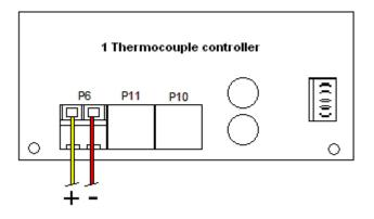
AF4X Kiln Controller Appendix F – Typical Wiring Diagram, 2 Heaters
